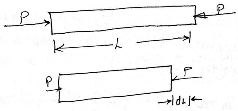
Let an axial push  $P$  is acting on a body of cross-sectional area  $A$ . Due to external push  $P$ , let the original length  $L$  of the body decreases by  $dl$ .
