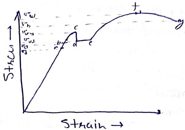
Point b :- This point is called elastic limit point. The stress corresponding to this point is called elastic limit ( $\sigma_e$ ) stress. There is a limiting value of force up to which within which, the deformation completely disappears on the removal of force. The value of stress corresponding to this limiting force is known as elastic limit of the material.
