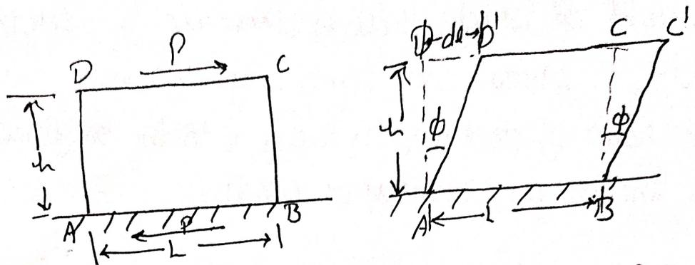
For the equilibrium of the block, the surface  $AB$  will offer a tangential reaction  $P$  equal & opposite to applied tangential force  $P$ .
