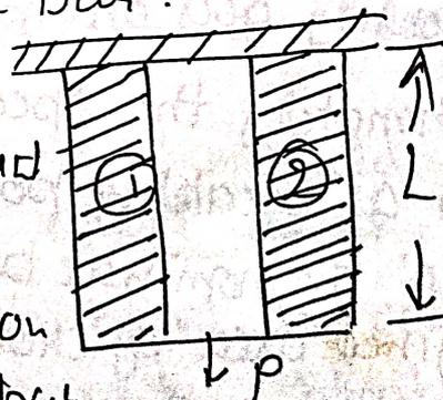
1. The extension or compression in each bar is equal. Hence deformation per unit length i.e. strain in each bar is equal.  $\epsilon_1 = \epsilon_2$
